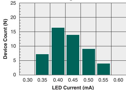
Typical  $I_F$  for Switch Dropout
