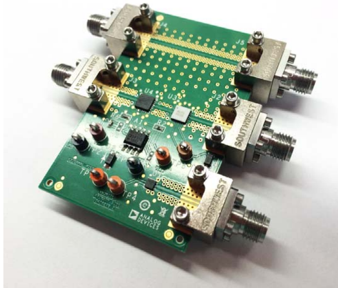
Figure 2. EVAL-CN0390-EB1Z AGC Printed Circuit Board (PCB) Photo
