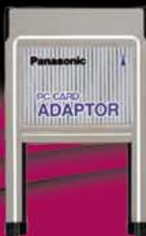
PC Card Adapter for Small PC Cards
