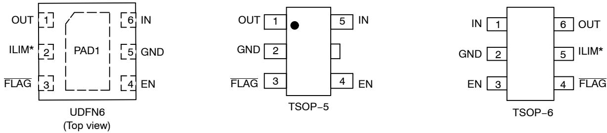
**Figure 2. Pin Connections**
