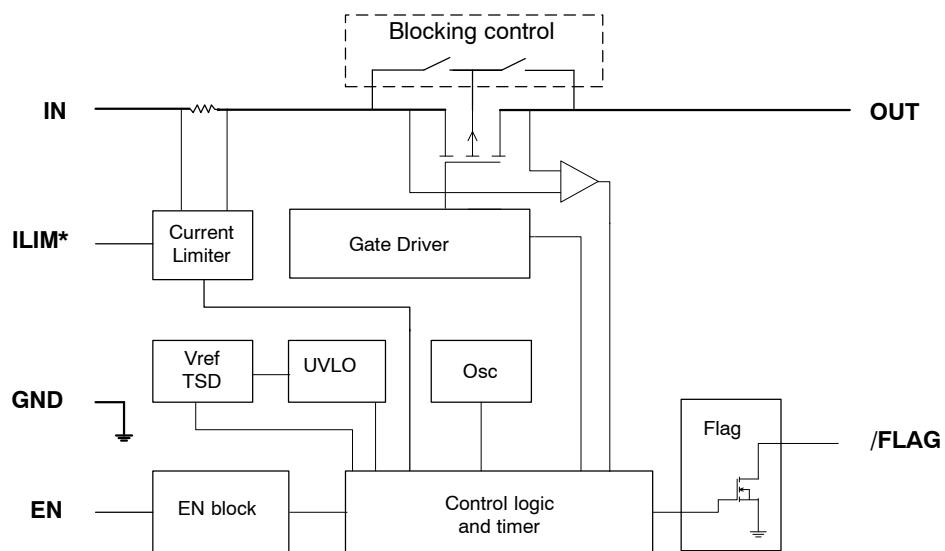
Figure 5. Block Diagram
