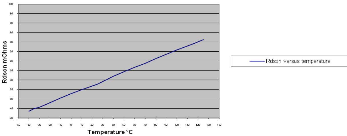
**Figure 21.**  $R_{DS(on)}$  vs Temperature,  $\mu$ DFN Package
