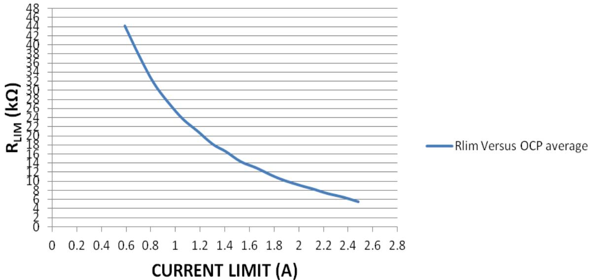
**Figure 25. R<sub>lim</sub> Curve versus Current Limit**
