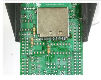
Finish up the resistors by placing  $\bf R8$  (100Kohm), and  $\bf R7$  (1.5K)
