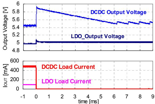
60) DC/DC Load Transient Response, LDO Output Voltage
