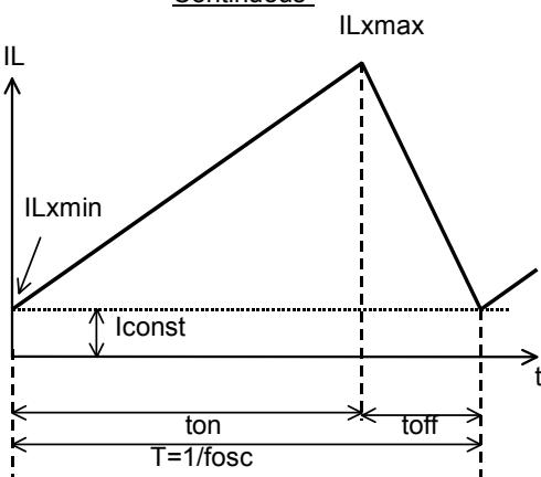
There are two modes, or discontinuous mode and continuous mode for the PWM step-up switching regulator depending on the continuous characteristic of inductor current. During on time of the transistor, when the voltage added on to the inductor is described as  $V_{IN}$ , the current is  $V_{IN} \times t/L$ . Therefore, the electric power,  $P_{ON}$ , which is supplied with input side, can be described as in next formula.
