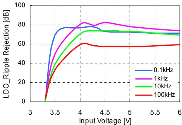
**35) LDO Ripple Rejection vs. Frequency**
