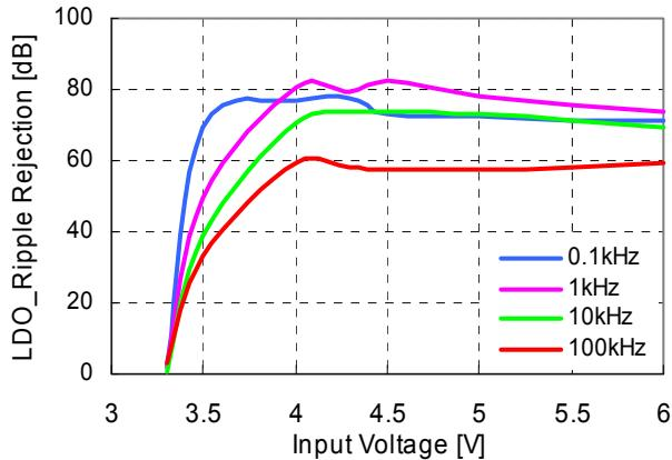
**35) LDO Ripple Rejection vs. Frequency**
