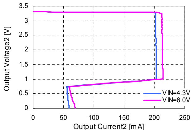
**25) Output Voltage 2 vs. Input Voltage**
