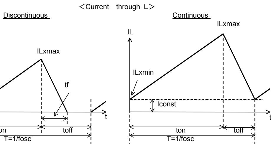
There are two modes, or discontinuous mode and continuous mode for the PWM step-up switching regulator depending on the continuous characteristic of inductor current. During on time of the transistor, when the voltage added on to the inductor is described as  $V_{IN}$ , the current is  $V_{IN}xt/L$ . Therefore, the electric power,  $P_{ON}$ , which is supplied with input side, can be described as in next formula.
