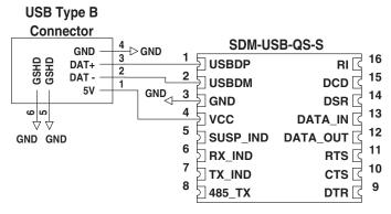
Figure 9: USB Bus-Powered Schematic
