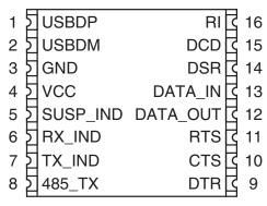
Figure 5: SDM-USB-QS-S Pinout (Top View)
