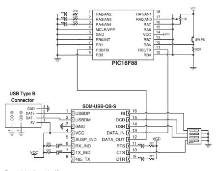
Figure 14: Interface with a Microprocessor
