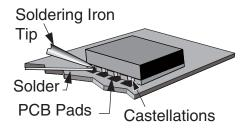
Figure 15: Soldering Technique
