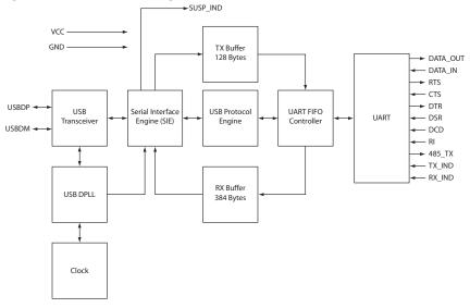
Figure 7: SDM-USB-QS-S Block Diagram
