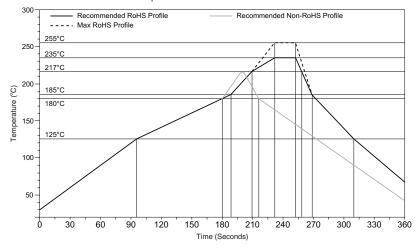
Figure 17: Maximum Reflow Temperature Profile
