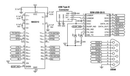
Figure 12: RS-232 to USB Converter
