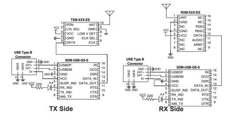
Figure 13: Wireless Modem Using ES Series RF Modules
