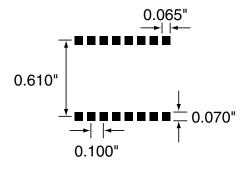
Figure 10: Recommended PCB Layout
