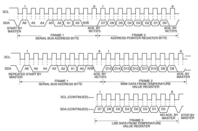
Figure 10. Typical Pointer Set followed by Two Bytes Register Read
