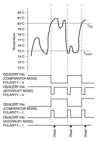
Figure 4. One-shot OS/ALERT Pin Operation
