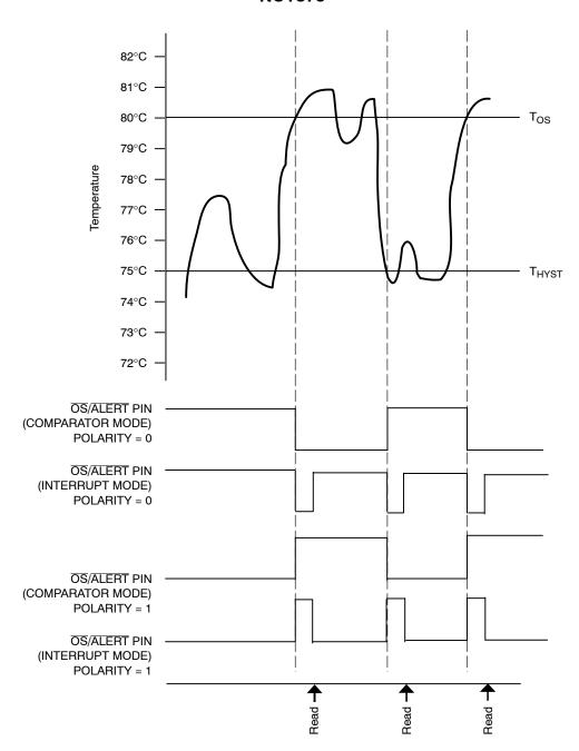
Figure 11. OS/ALERT Output Temperature Response Diagram
