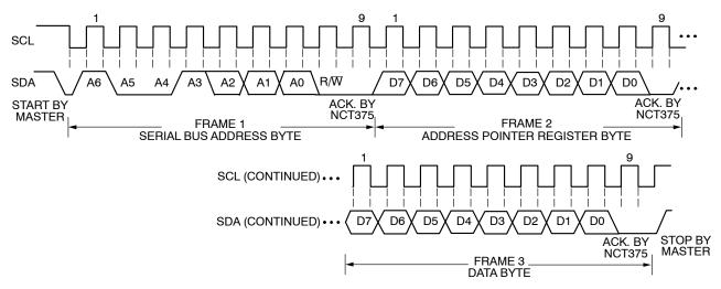
Figure 6. Writing a Register Address to the Address Pointer Register, then Writing a Single Byte of Data to the Configuration Register
