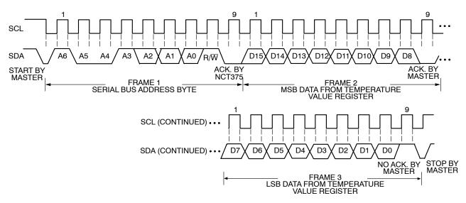
Figure 9. Reading Data from the Temperature Value Register with Preset Pointer Register
