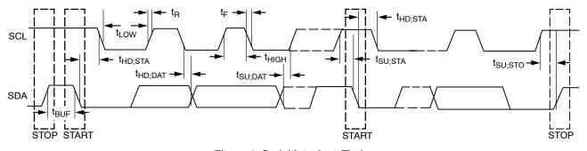
Figure 3. Serial Interface Timing
