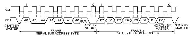
Figure 8. Reading Data from the Configuration Register
