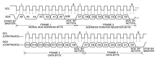
Figure 7. Writing to the Address Pointer Register Followed by Two Bytes of Data to a 16 Bit Limit Register
