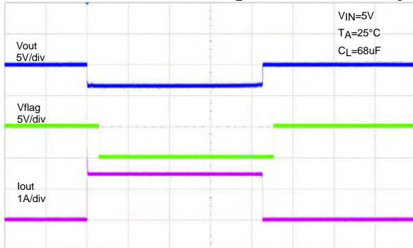
Short Circuit with Blanking Time and Recovery
