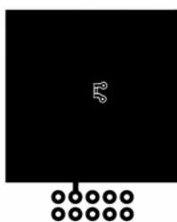
a. 60 °C/W when mounted on a 1 in<sup>2</sup> pad of 2 oz copper.
