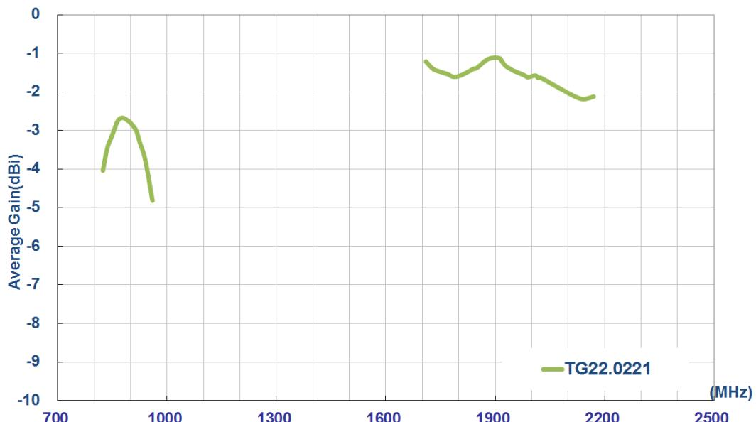
Figure 5. Average Gain of the TG.22 Antenna.
