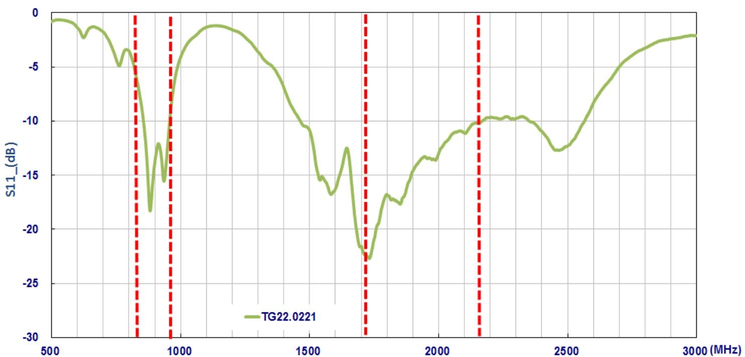
**Figure 2.** Return loss of the TG.22 antenna.
