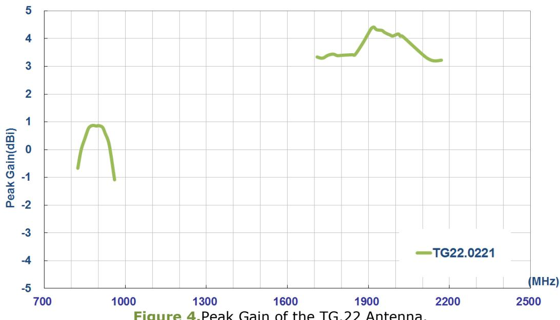
Figure 4. Peak Gain of the TG.22 Antenna.
