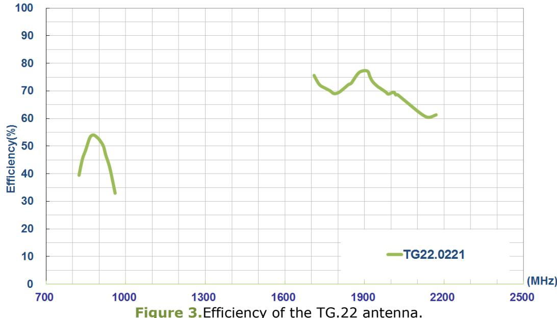
Figure 3. Efficiency of the TG.22 antenna.
