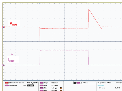
Figure 24. Load transient ( V_{IN} = V_{EN} = 3.5\text{ V} ; t_{RISE} = 1\text{ }\mu\text{s} ; I_{OUT} = 1\text{ mA} to 1\text{ A} )
