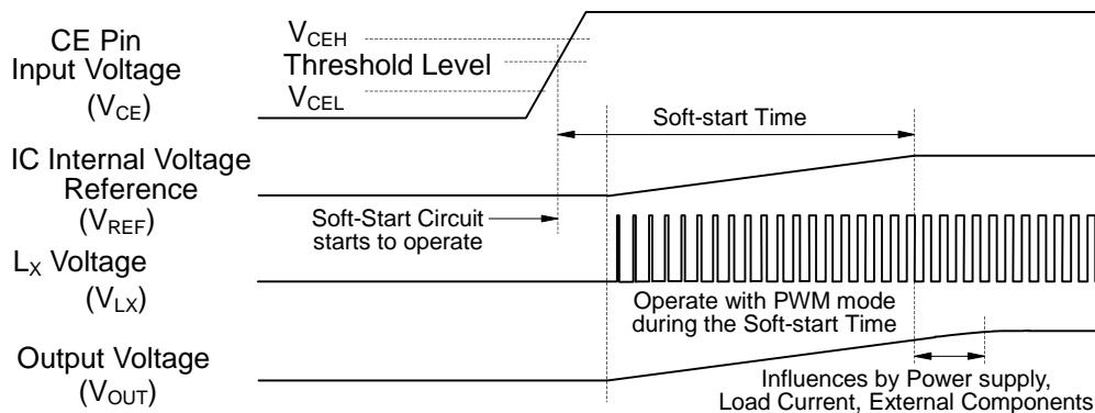
Soft-start time is the time period from when the soft-start circuit started to when the reference voltage reached to the specified value.
