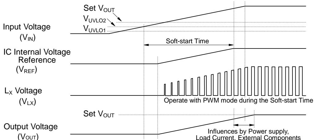
\*The start-up speed of the output voltage could be affected by the following elements.
