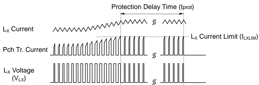
To release the latch type protection circuit, reset the ICs by inputting "L" into CE pin or make the input voltage lower than the UVLO detector threshold ( $V_{UVLO1}$ ).
