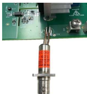
Figure 15. SDN-414-01 current viewing resistor (sold separately)
