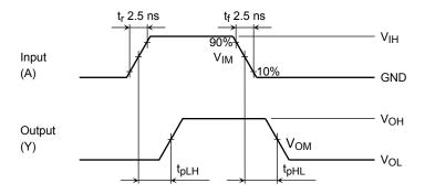
Figure 2 t<sub>pLH</sub>, t<sub>pHL</sub>
