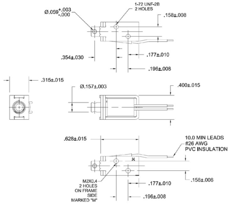
Solenoid shown energized with plunger fully seated
