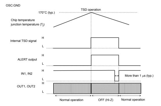
Note: The TSD circuit is activated if the absolute maximum junction temperature rating  $(T_j)$  of 150°C is violated. Note that the circuit is provided as an auxiliary only and does not necessarily provide the IC with a perfect protection from any kind of damages.
