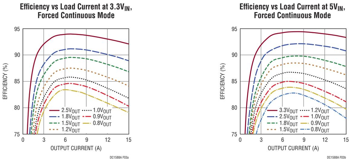
Figure 2. Measured Supply Efficiency with Different V<sub>IN</sub> and V<sub>OUT</sub>
