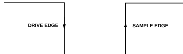
Figure 66. SPI Mode 3, SCLK Edges
