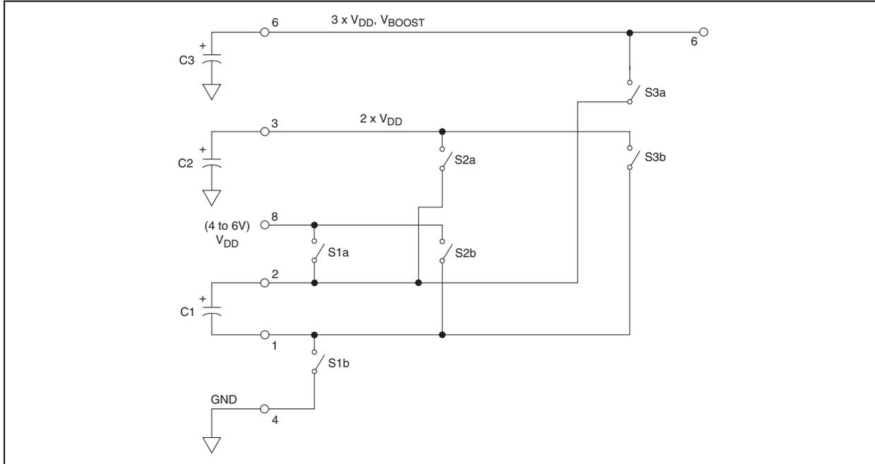
**FIGURE 3-4: POSITION OF SWITCHES**
