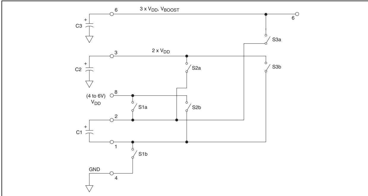
**FIGURE 3-4: POSITION OF SWITCHES**
