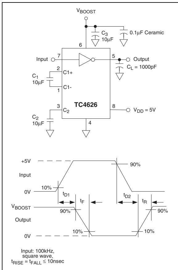
**FIGURE 3-2:** NONINVERTING DRIVER
