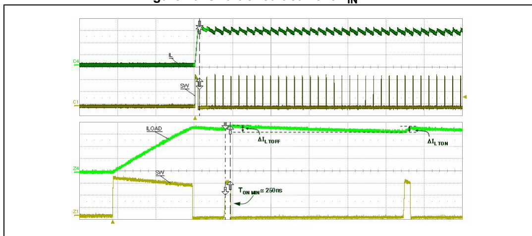
Figure 20. Short-circuit current V_{IN} = 24\text{ V}
