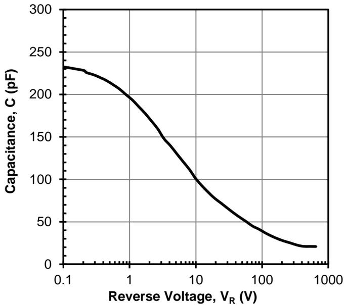
**Figure 7** Capacitance vs. reverse voltage at 1MHz
