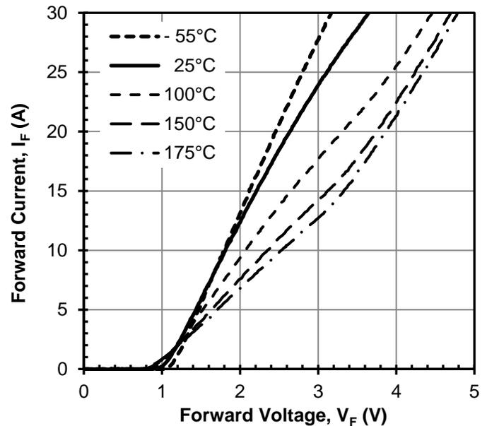
Figure 2 Typical forward characteristics in surge current
