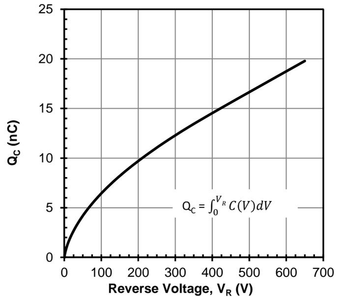
**Figure 8** Typical capacitive charge vs. reverse voltage
