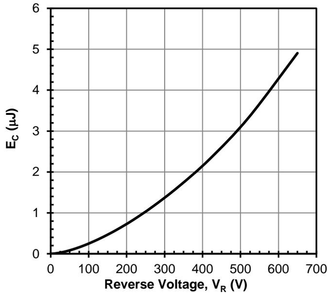
**Figure 9** Typical capacitance stored energy vs. reverse voltage
