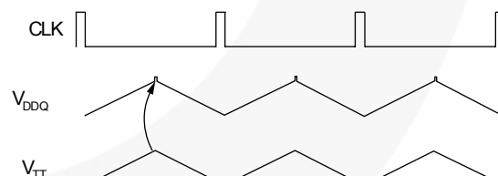
Figure 9. Noise-Susceptible In-Phase Operation for DDR2
