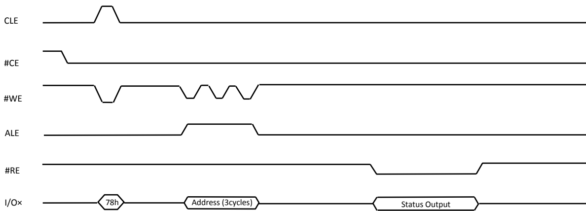
Figure 9-11 Read Status Enhanced (78h) Operation
