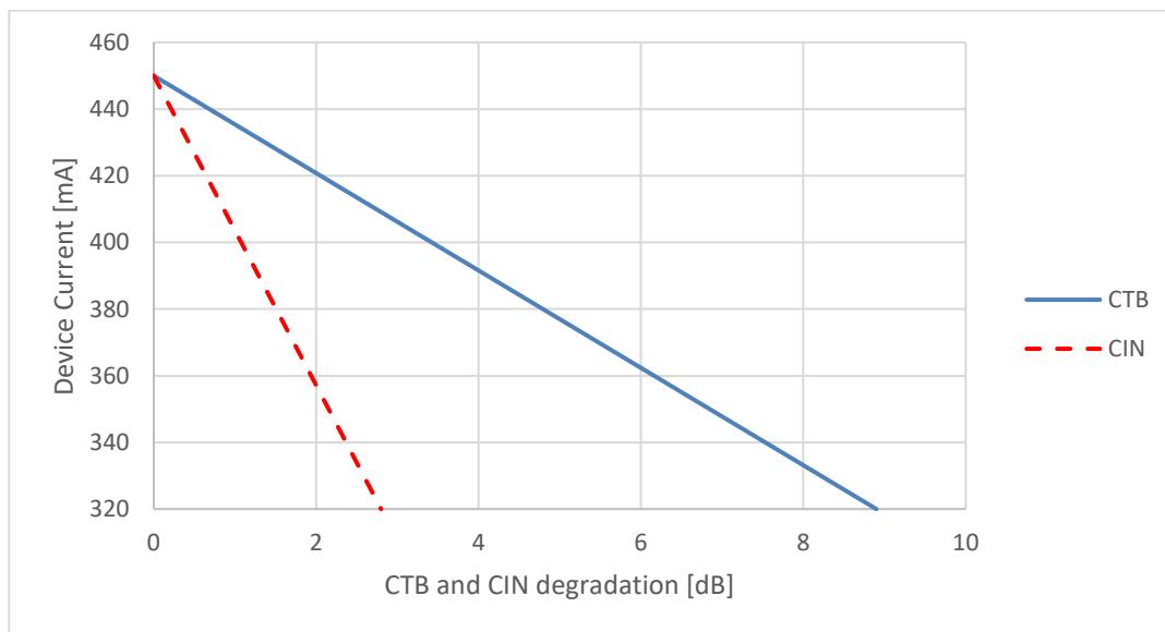
Test Condition: V+=24V, TMB=30°C, ZS=ZL=75Ω, IDC=IDC (typ.), NTSC, 79ch analog: 48.5dBmV @ 547.25 MHz; 7 dB tilt, with 111 J.83/B QAM256 channels (6 dB down)
