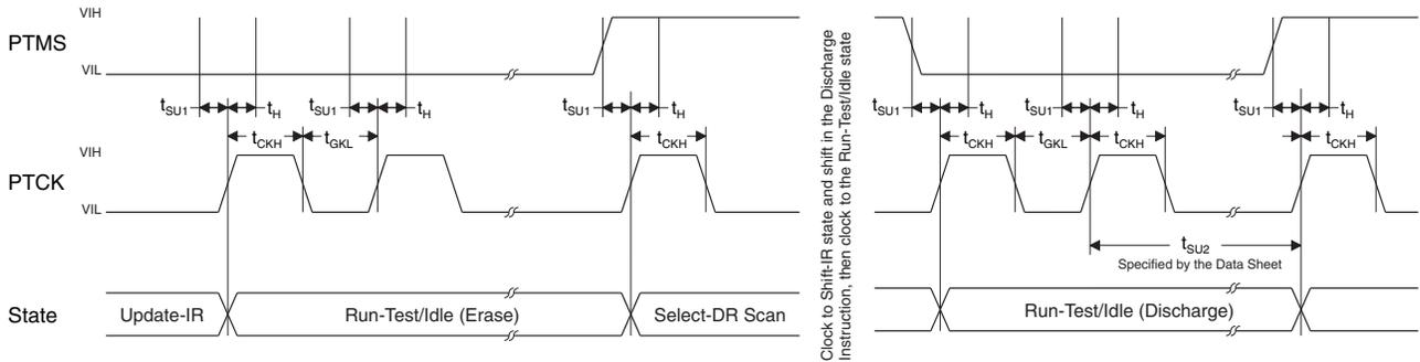
Figure 8. Programming Timing Diagram
