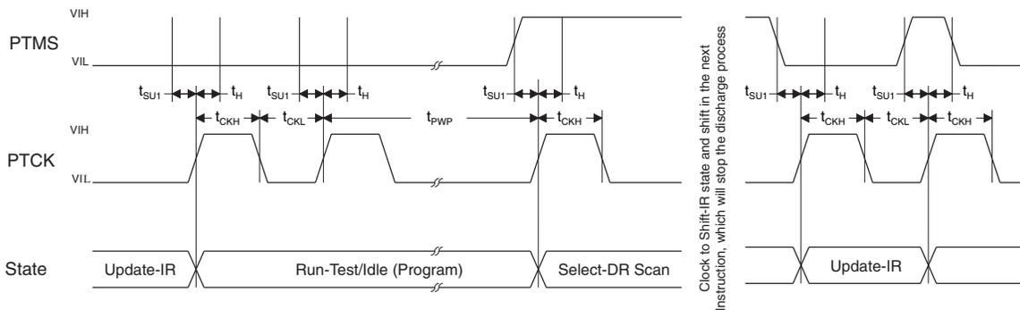
**Figure 9. Verify Timing Diagram**
