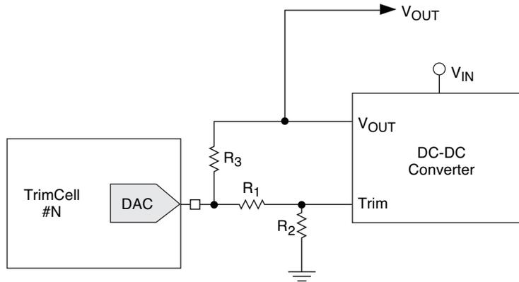
Figure 17 shows the resistor network between the TrimCell #N in the Platform Manager and the DC-DC converter. The values of these resistors depend on the type of DC-DC converter used and its operating voltage range. The method to calculate the values of the resistors R1, R2, and R3 are described in a separate application note.
