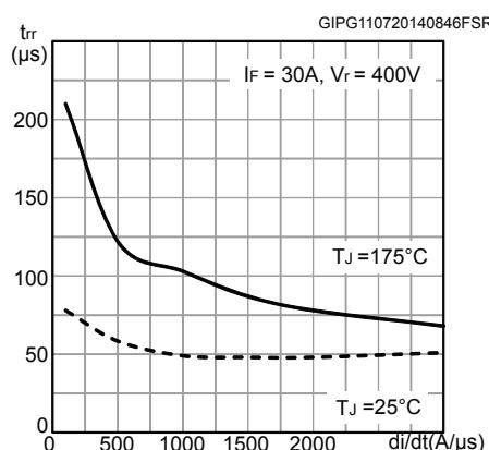
**Figure 23. Reverse recovery charge vs diode current slope**
