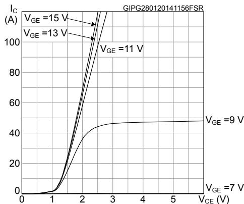
**Figure 4. Output characteristics ( $T_J = 175 \text{ °C}$ )**
