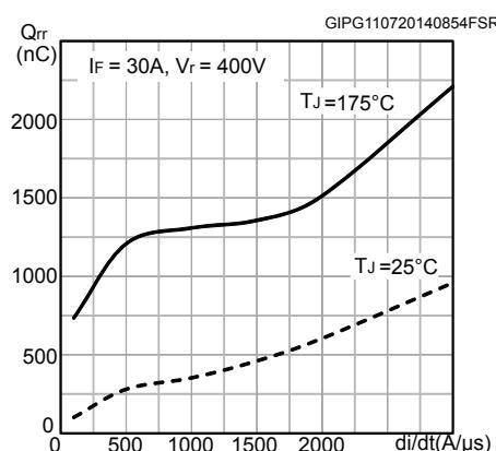
**Figure 24. Reverse recovery energy vs diode current slope**
