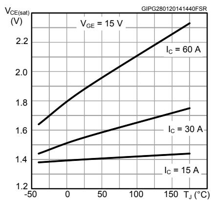
**Figure 6.  $V_{\text{CE}(\text{sat})}$  vs collector current**
