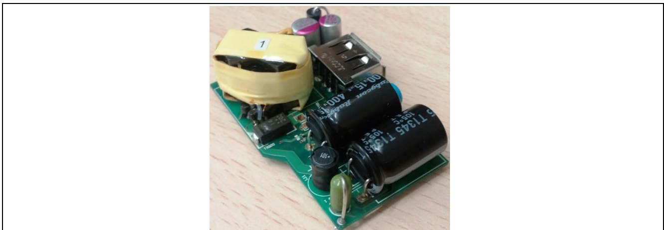
Figure 1 REF-15W_C61K5-THINPAK ADAPTER [Dimensions L x W x H: 47mm x 31mm x 16mm]
