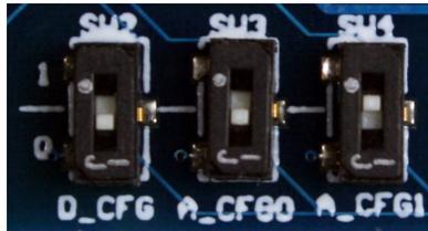
Figure 7: The Evaluation Board Input Interpretation Selection Switches
