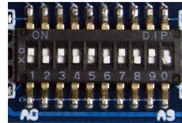
Figure 5: The Evaluation Board Address DIP Switch
