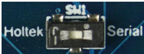
Figure 8: The Evaluation Board Protocol Selection Switch
