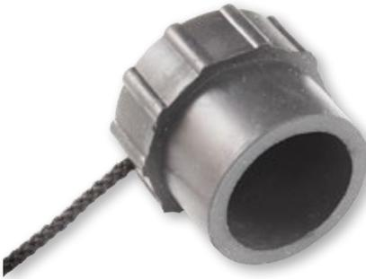
These *splashproof molded rubber covers* fit all Series 801 plugs and receptacles. Braided black nylon lanyard is available with metal rings, cable tie or slipknot for attachment to panel or to cable. -40° to +120° C operating temperature, fungus resistant per MIL-STD-810G Method 508.6.
