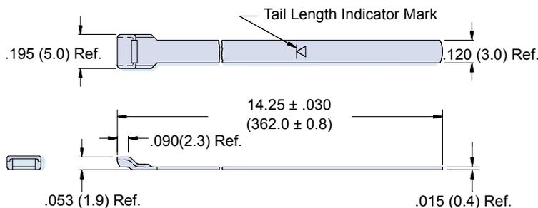
**The 600-083 Extended Length Micro-Band** is precision constructed of 300 Series SST/Passivate, and designed for use with the 600-061 Hand Banding Tool or the 600-068 Pneumatic Banding Tool. Double-wrapped bands will accommodate diameters up to approximately 1.88 inches (47.8). Bands may be ordered flat (600-083), or precoiled (600-083-1). Bands come bagged and tagged in quantities from 1 to 100.
