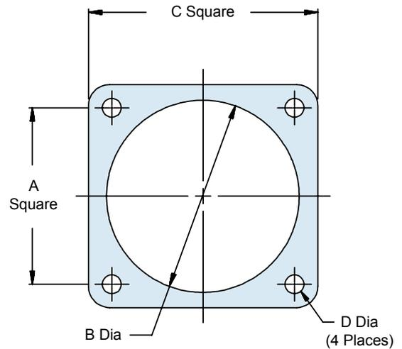
**Commercial equivalent square flange wall mount receptacle panel gasket**
