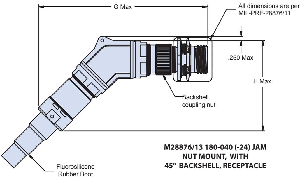
**M28876/13 180-040 (-24) JAM NUT MOUNT, WITH 45° BACKSHELL, RECEPTACLE**
