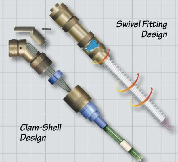
*The fiber optic backshell pictured above on the left features a unique "clam shell" opening, as well as a tensioning device to prevent overtightening of the backshell clamp. The assembly pictured on the right features a unique swivel fitting to prevent cable torque from affecting fiber alignment. Both are suited for use with standard extruded cable or conduit.*
