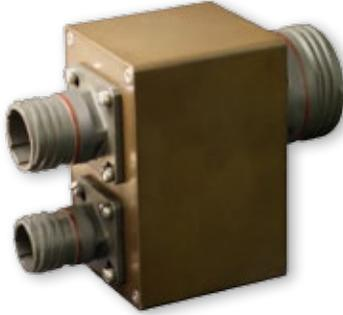
The Glenair Gigabit Ethernet Media Converter is mechanically hardened to resist weapon-grade shock and vibration benchmarks and is environmentally sealed to IP68 when connectors are in their mated condition. The device is equipped with a gigabit physical layer transceiver to convert electrical data to a standardized serial format and an optical transceiver for electrical to F/O conversion.
