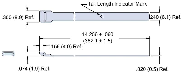
**The 600-052 Standard Band** is precision constructed of 300 Series SST/Passivate and designed for use with the 600-058 Hand Banding Tool or the 600-067 Pneumatic Banding Tool. Double-wrapped bands will accommodate diameters up to approximately 1.8 inches (45.7). Bands may be ordered flat (600-052) or precoiled (600-052-1). Bands come bagged and tagged in quantities from 1 to 100.
