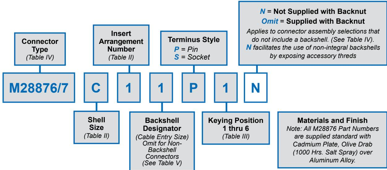
Glenair commercial equivalent MIL-PRF-28876 type fiber optic connectors
