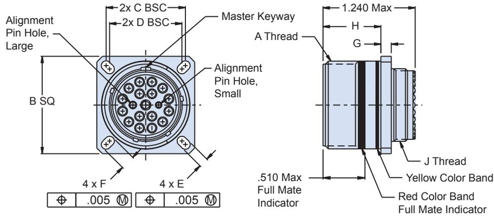
**S7 - Wall Mount Receptacle with Slotted Holes**
