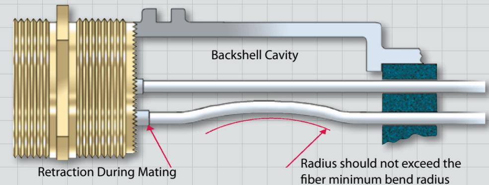
cable to insure the best possible fiber position and alignment.
