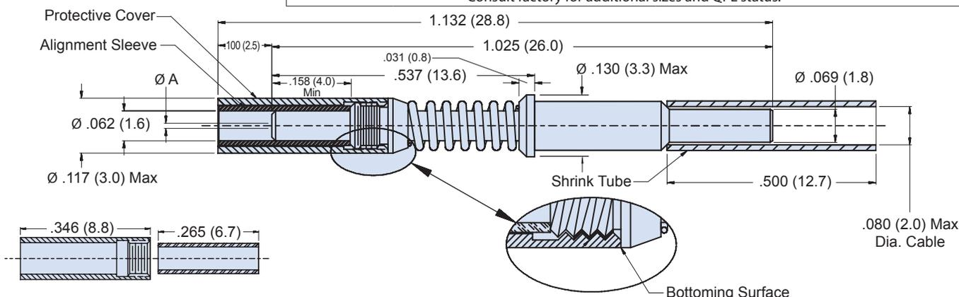
Ceramic alignment sleeve supplied with terminus. Add K to the end of part number development to supply with optional stainless steel alignment sleeve e.g. 181-001-126K.
