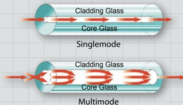
Singlemode fibers are manufactured with the smallest core size (approximately 8 - 10 um in diameter) and so they eliminate modal dispersion by forcing the light pulses to follow a single, direct path. The bandwidth of a singlemode fiber so far surpasses the capabilities of multimode fiber that its information-carrying capacity is essentially infinite. Singlemode fiber is thus the preferred medium for long distance and high bandwidth applications.
