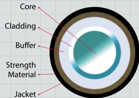
reflection possible, as the difference in materials used in the core and the cladding creates an extremely reflective surface at the point where they interface. Light pulses entering the fiber core reflect off the core/cladding interface and thus remain within the core as they move down the line.
