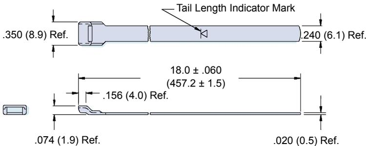
**The 600-090 Extended Length Standard Band** is precision constructed of 300 Series SST/Passivate, and designed for use with the 600-058 Hand Banding Tool or the 600-067 Pneumatic Banding Tool. Double-wrapped bands will accommodate diameters up to approximately 2.5 inches (63.5). Bands may be ordered flat (600-090), or precoiled (600-090-1). Bands come bagged and tagged in quantities from 1 to 100.
