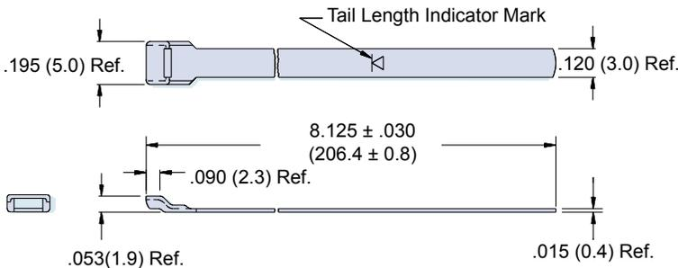
**The 600-057 Micro Band** is precision constructed of 300 Series SST/Passivate, and designed for use with the 600-061 Hand Banding Tool or the 600-068 Pneumatic Banding Tool. Double-wrapped bands will accommodate diameters up to approximately .88 inches (22.4). Bands may be ordered flat (600-057), or precoiled (600-057-1). Bands come bagged and tagged in quantities from 1 to 100.
