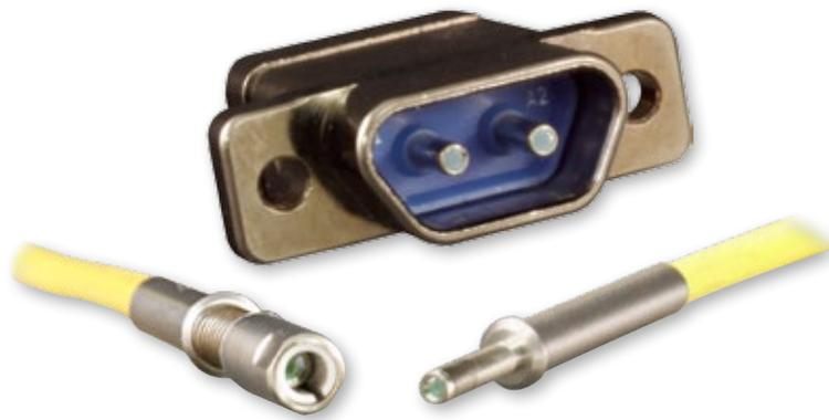
Eye-Beam™ Expanded Beam fiber optic terminus can be integrated into virtually any circular or rectangular connector package. Factory terminated lens pin terminus and lens socket terminus on cable jumpers allow for easy fusion splicing in the field.
