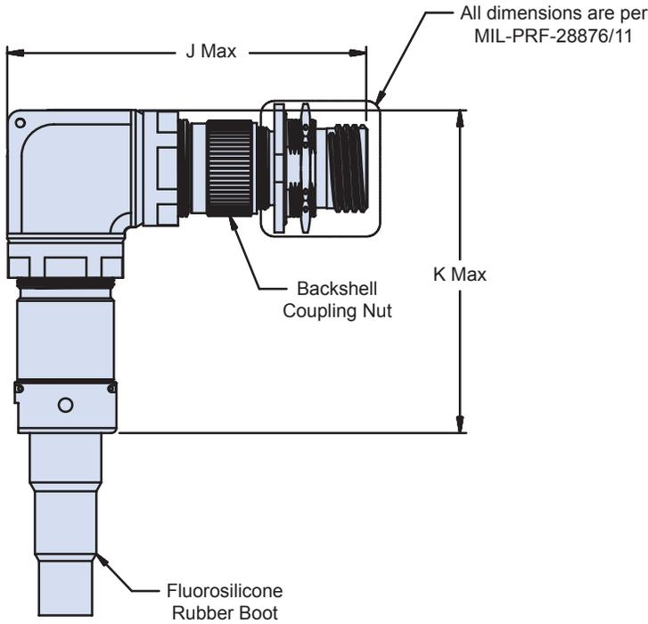
**M28876/14 180-040 (-34) JAM NUT MOUNT, WITH 90° BACKSHELL, RECEPTACLE**
