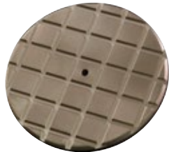
Polishing Puck showing grooves for wet polish
