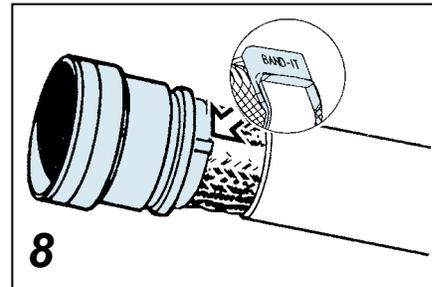
5. Aligning the Band and Tool with the Shield Termination Area, squeeze Black Pull-Up Handle repeatedly using short strokes until it locks against Tool Body. (This indicates the Band is compressed to the Tool Precalibrated Tension.)
