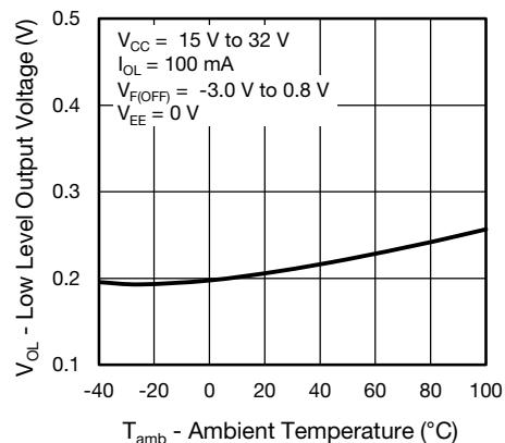
Fig. 8 - Low Level Output Voltage vs. Ambient Temperature
