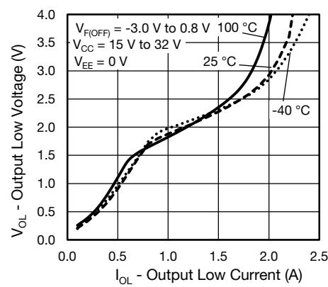
Fig. 10 - Output Low Voltage vs. Output Low Current
