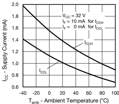
Fig. 12 - Supply Current vs. Ambient Temperature
