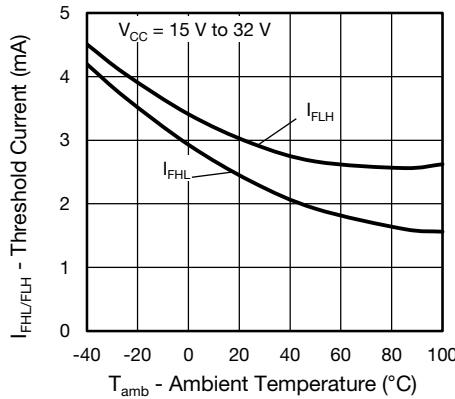
Fig. 14 - threshold Current vs. Ambient Temperature
