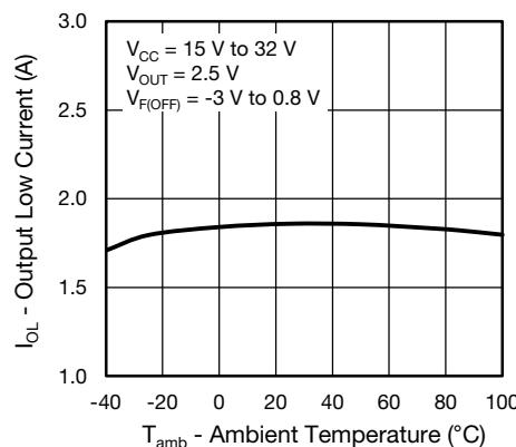
Fig. 9 - Output Low Current vs. Ambient Temperature
