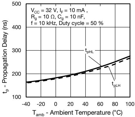
Fig. 17 - Propagation Delay vs. Ambient Temperature
