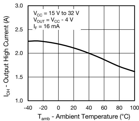
Fig. 7 - Output High Current vs. Ambient Temperature
