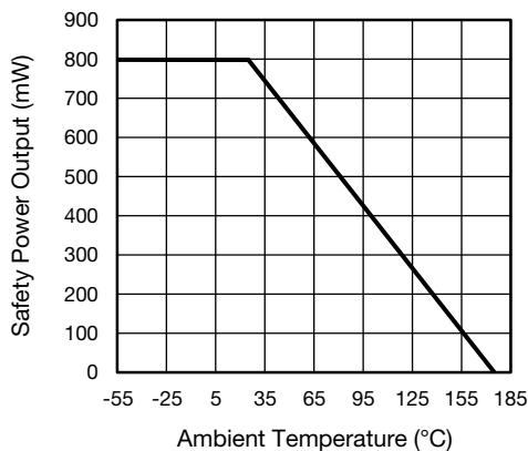
Fig. 4 - Safety Power Dissipation vs. Ambient Temperature
