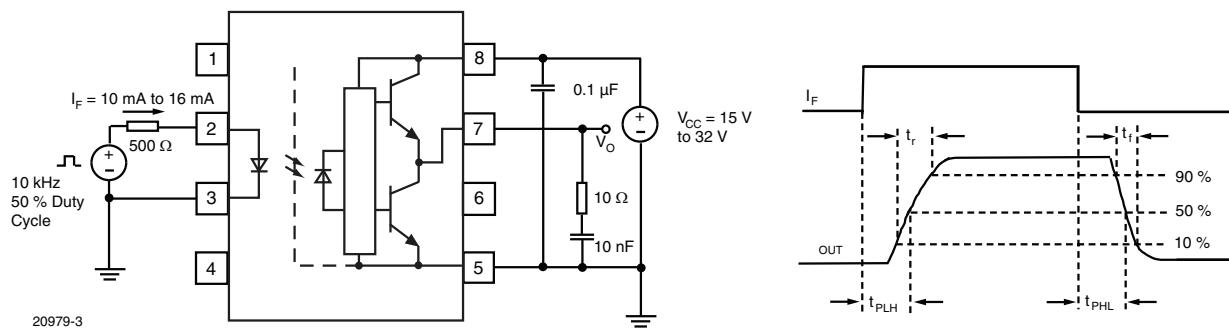
Fig. 2 -  $t_{PLH}$ ,  $t_{PHL}$ ,  $t_r$  and  $t_f$  Test Circuit and Waveforms
