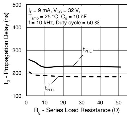
Fig. 19 - Propagation Delay vs. Series Load Resistance
