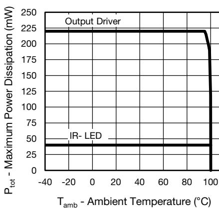
Fig. 1 - Dissipated Operating Power vs. Operating Temperature
