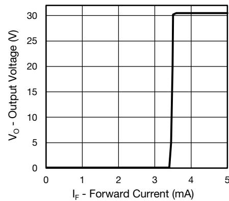
Fig. 15 - Output Voltage vs. Forward Current
