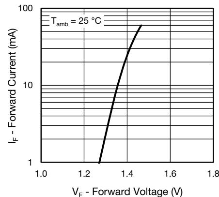
Fig. 21 - Forward Current vs. Forward Voltage
