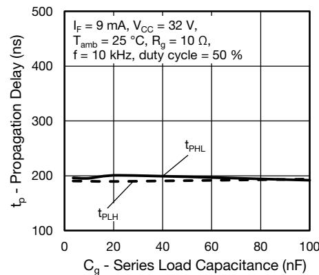
Fig. 20 - Propagation Delay vs. Series Load Capacitance
