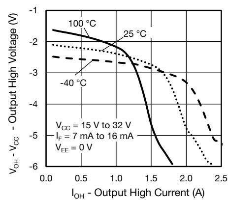
Fig. 11 - Output High Voltage vs. Output High Current
