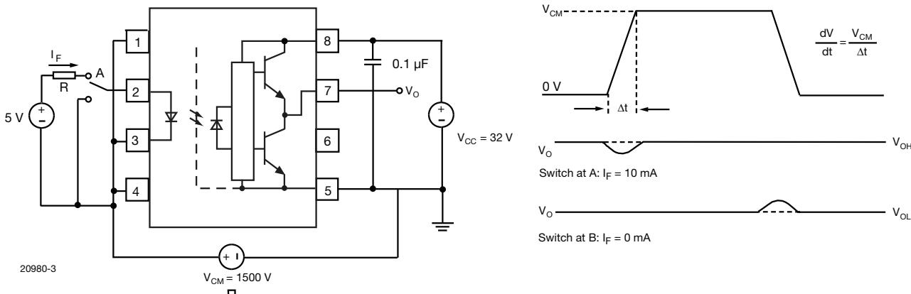
Fig. 3 - CMR Test Circuit and Waveforms
