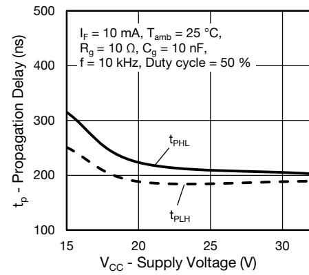
Fig. 16 - Propagation Delay vs. Supply Voltage
