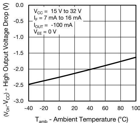
Fig. 6 - High Output Voltage Drop vs. Ambient Temperature
