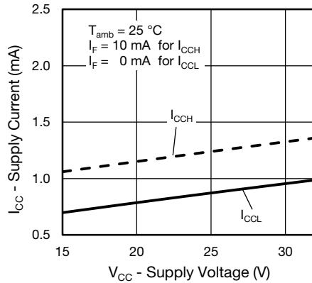
Fig. 13 - Supply Current vs. Supply Voltage
