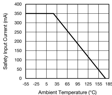
Fig. 5 - Safety Input Current vs. Ambient Temperature
