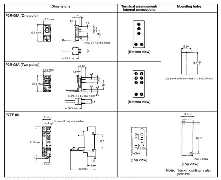
Note: When indicator modules with an I/O SSR are used, the No. 1 pin becomes positive.
