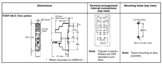
Note: When indicator modules with an I/O SSR are used, the No. 1 pin becomes positive.
