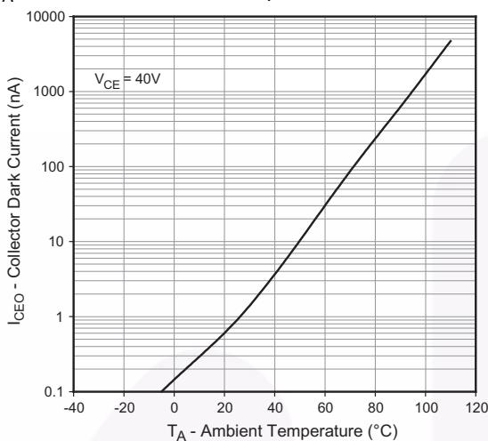
**Fig. 9. Collector Dark Current vs. Ambient Temperature (FODM121/2701/2705)**
