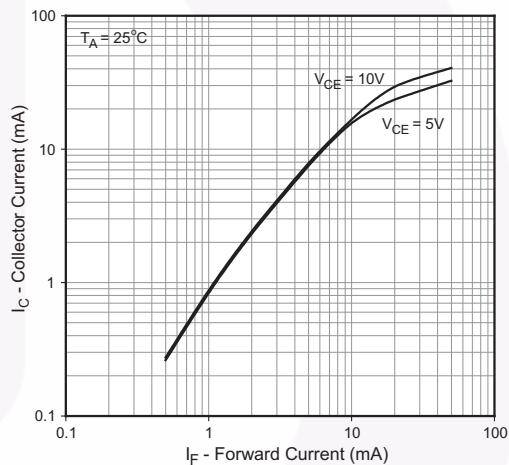
**Fig. 6 Collector Current vs. Forward Current (FODM121/2701/2705)**
