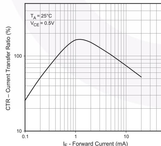
**Fig. 13 Current Transfer Ratio vs. Forward Current (FODM124)**
