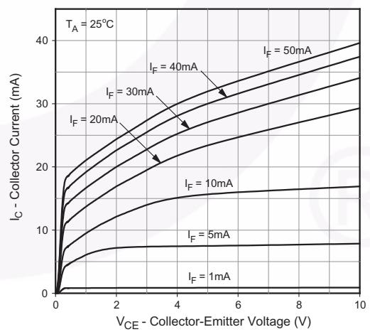
**Fig. 8 Collector Current vs. Collector-Emitter Voltage (FODM121/2701/2705)**
