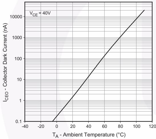
**Fig. 17 Collector Dark Current vs. Ambient Temperature (FODM124)**
