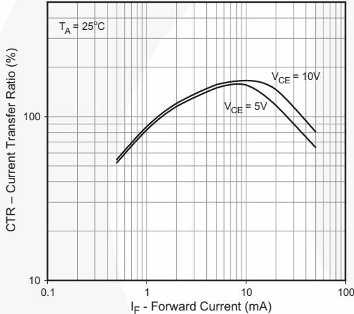
**Fig. 5 Current Transfer Ratio vs. Forward Current (FODM121/2701/2705)**
