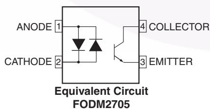
Figure 1. Schematic
