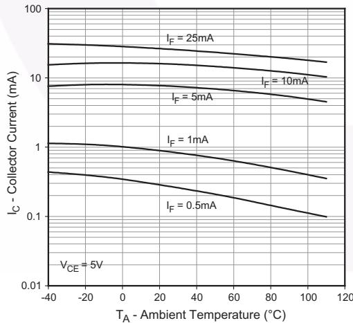
**Fig. 7 Collector Current vs. Ambient Temperature (FODM121/2701/2705)**
