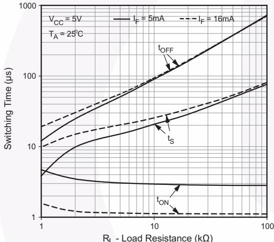
**Fig. 11 Switching Time vs. Load Resistance (FODM121/2701/2705)**
