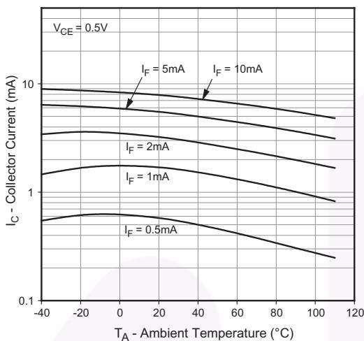
**Fig. 15. Collector Current vs. Ambient Temperature (FODM124)**
