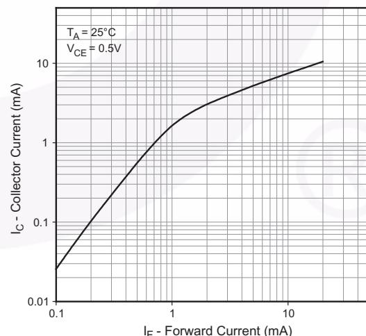
**Fig. 14. Collector Current vs. Forward Current (FODM124)**
