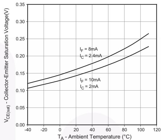
**Fig. 4 Collector-Emitter Saturation Voltage vs. Ambient Temperature (FODM121/2701/2705)**
