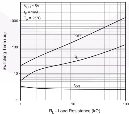
**Fig. 19 Switching Time vs. Load Resistance (FODM124)**
