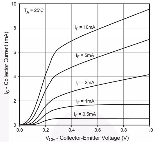
**Fig. 16 Collector Current vs. Collector-Emitter Voltage (FODM124)**
