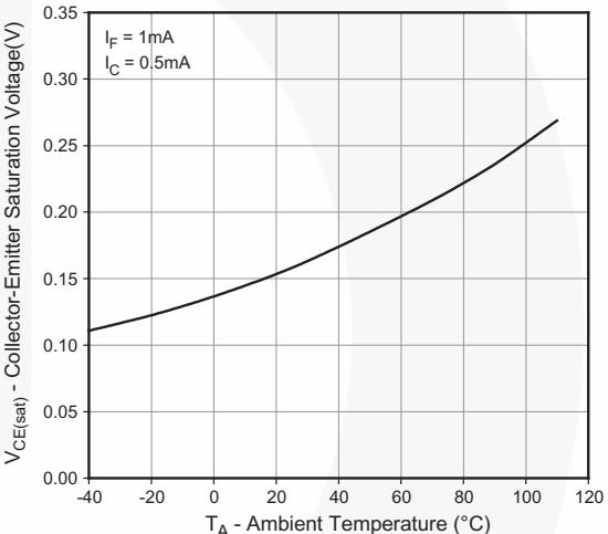
**Fig. 12 Collector-Emitter Saturation Voltage vs. Ambient Temperature (FODM124)**
