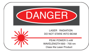
Figure 5. Warning logotype label for Class IIIa lasers.
