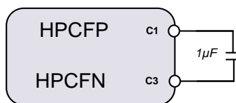
Figure 41: Charge Pump Flying Capacitor
