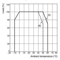
**Note:** The derating curve depends on the mounting direction of the Power Supply
