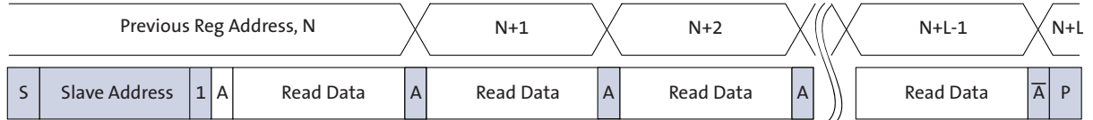
Figure 23: Sequential READ, Start from Current Location
