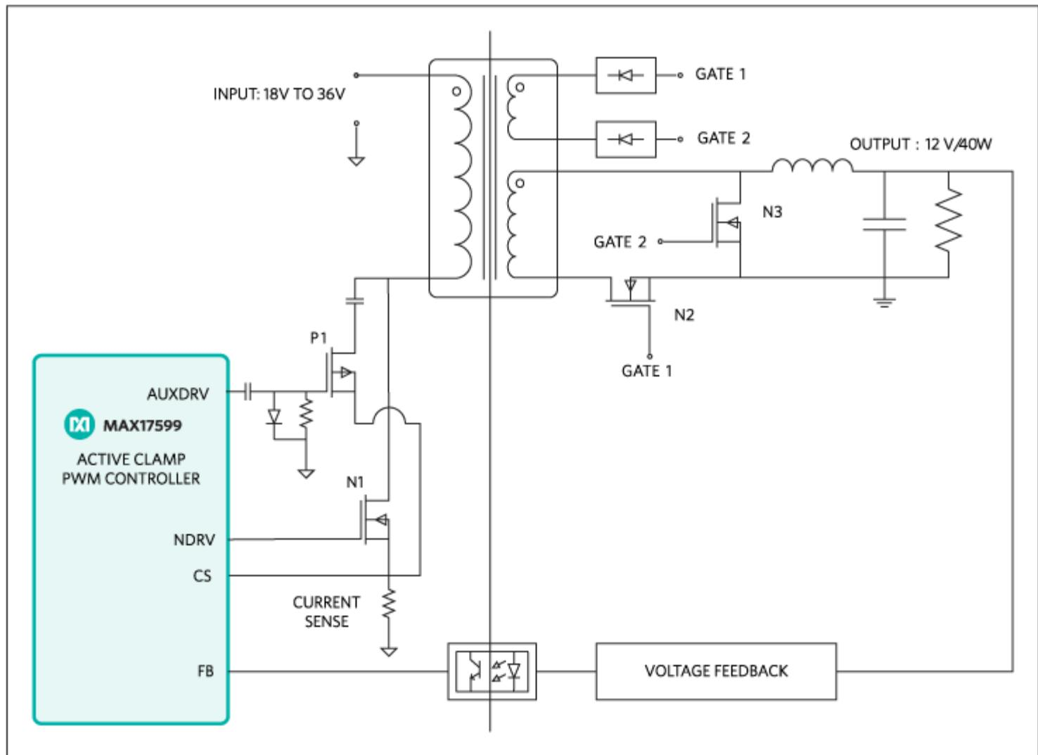
Figure 1. The MAXREFDES48# reference design block diagram.
