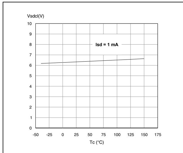
**Figure 30. High level STAT\_DIS voltage**
