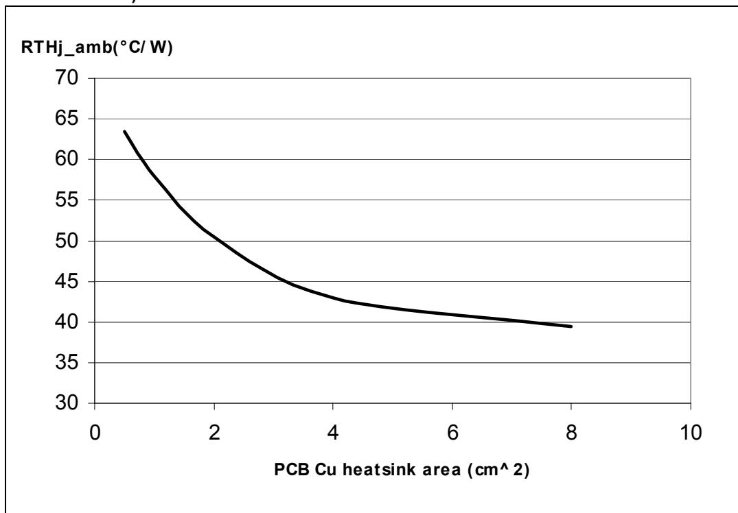
**Figure 37. PowerSSO-12 thermal impedance junction ambient single pulse (one channel on)**
