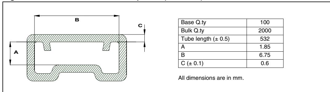
**Figure 46. PowerSSO-12 tape and reel shipment (suffix "TR")**
