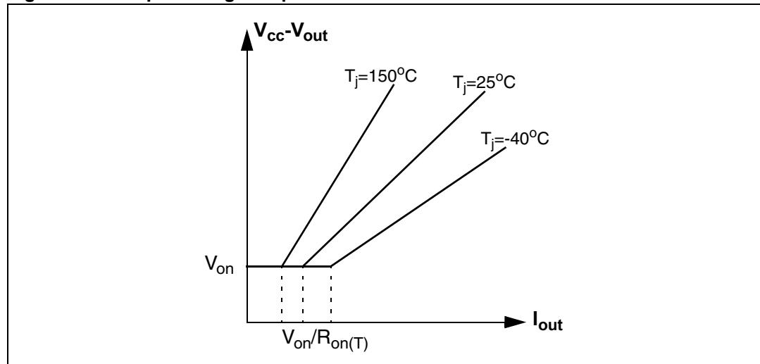
**Figure 6. Switching characteristics**
