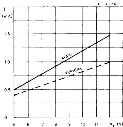
**Figure 18. Input current as a function of input voltage (for ULN2803A)**
