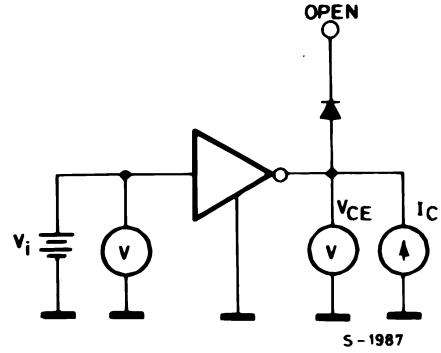
Figure 9. Clamp diode leakage current
