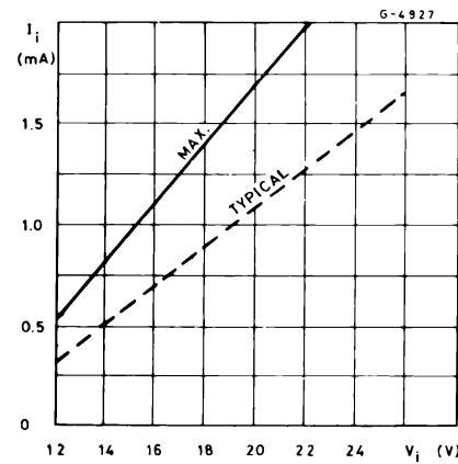
**Figure 17. Input current as a function of input voltage (for ULN2804A)**
