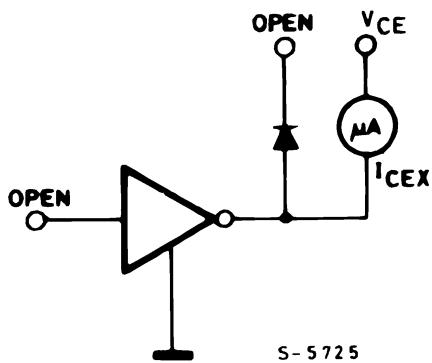
Figure 4. Output leakage current (for ULN2802A only)
