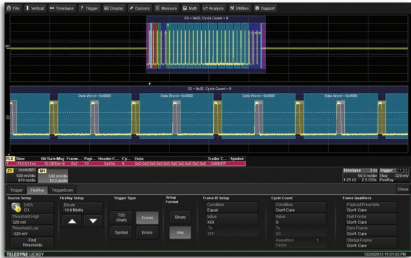
Trigger on every aspect of the FlexRay Frame as well as Symbols and Errors including FSS, BSS, FES, CRC, CID, CAS/MTS and Wakeup by selecting the appropriate boxes.
