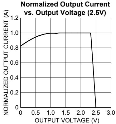
Figure 4. Normalized Output Current vs. Output Voltage
