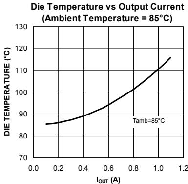
Figure 2. Die Temperature vs.  $I_{OUT}$
