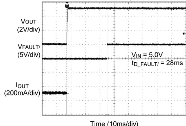
**2098 Output Recovery from Short Circuit and FAULT/Response**
