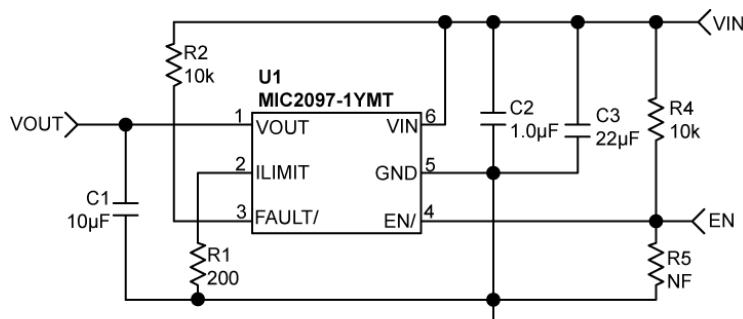
**Figure 8. MIC2097-1 Typical Schematic**
