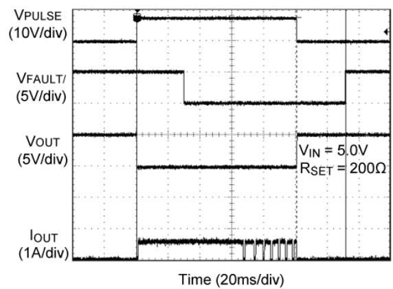
**2097 Output Recovery from Thermal Shutdown**
