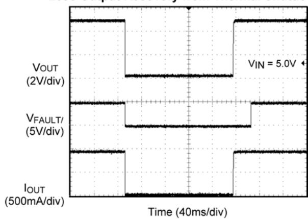
**2099 Output Recovery from Thermal Shutdown**
