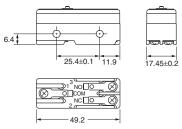
Note: Appropriate terminal screw tightening torque: 0.78 to 1.18 N·m.
