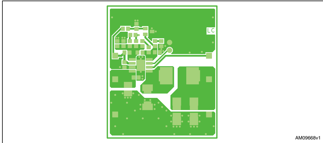
Figure 25. PCB layout (front side)
