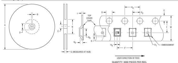
В D Ν G Min. Max. Min. Max. Min. Max. Min. Max. Ref. Ref. 328.5 331 2.0 2.4 12.8 13.5 17.0 17.4 16.5 100 ± 1.5 (0.669)(0.690)(12.93)(13.05)(0.079)(0.094)(0.504)(.531)(0.650) $(3.94 \pm 0.059)$
