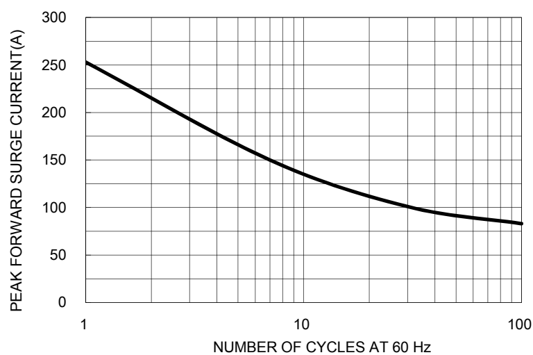
FIG. 3- MAXIMUM NON-REPETITIVE FORWARD SURGE CURRENT
