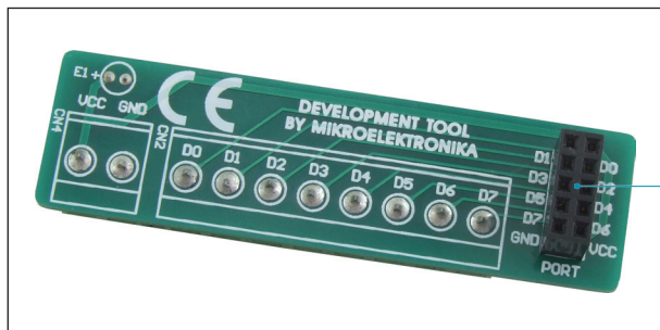
Figure 2: EasyConnect additional board's bottom view
