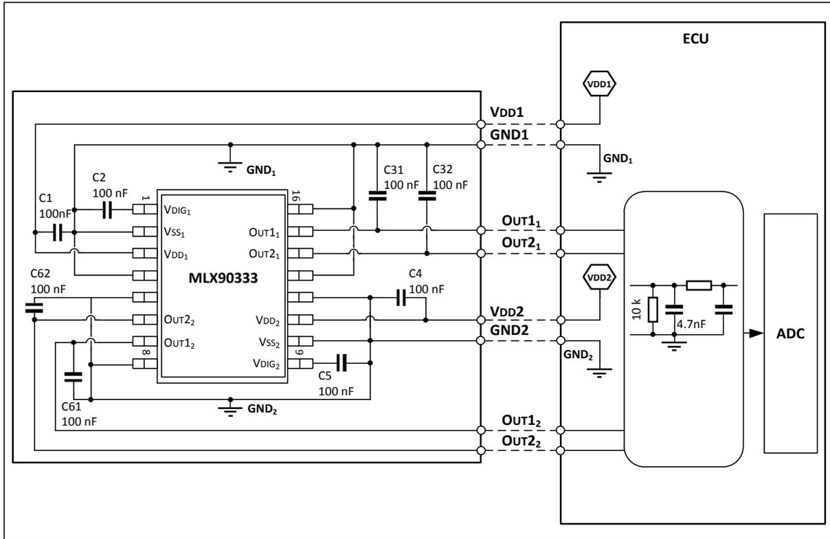
Figure 12 – Recommended wiring in TSSOP-16 package (dual die)
