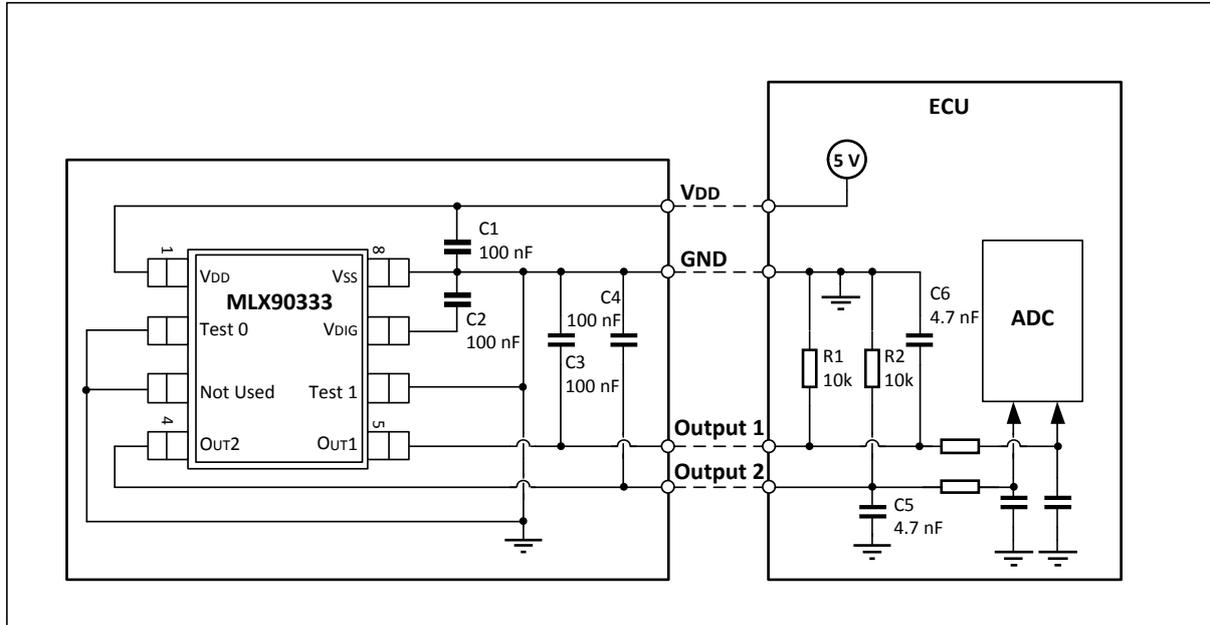
Figure 10 – Recommended wiring in SOIC-8 package
