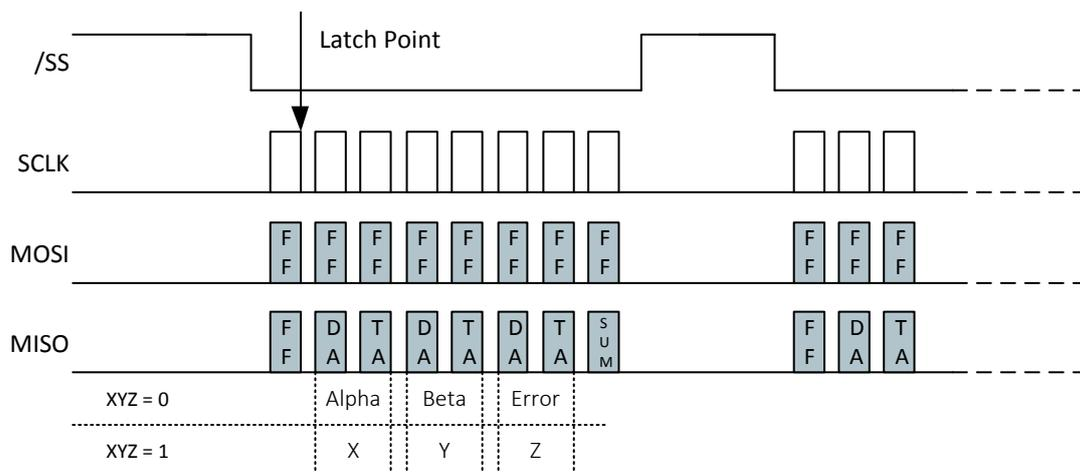
Figure 9 – Timing Diagram for the SPI Frame
