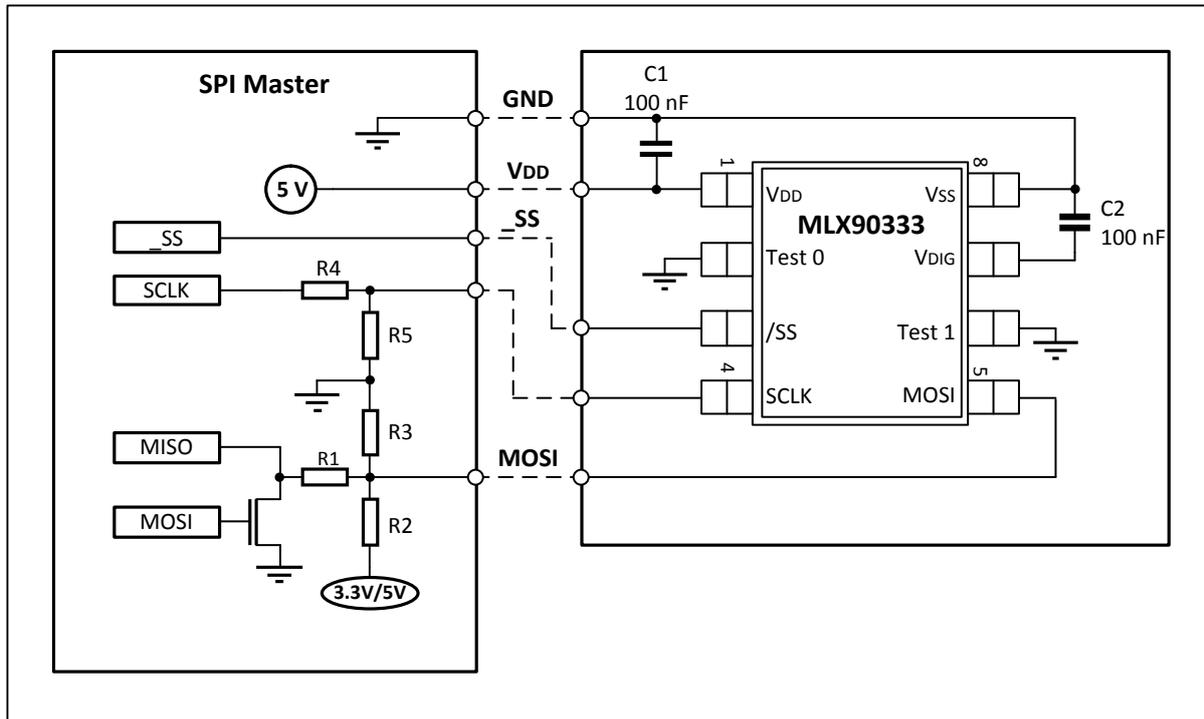
Figure 13 – SPI Version – Single Die – Application Diagram
